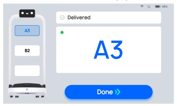
Step 6 Once the operator removes the item, tap "Complete," and the robot will then begin executing its next task. If the robot has completed all tasks, it will return to the docking point.
