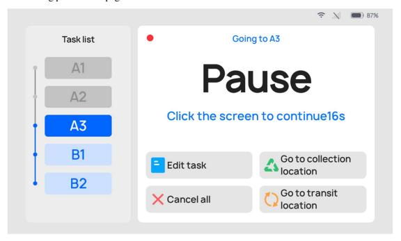
During the recycling process, if it is necessary to edit a task, go to collection point, cancel all tasks, or return, you can tap on the robot's screen to pause the robot before proceeding with the operation. If there are no operations during the countdown period, the robot will continue running.
