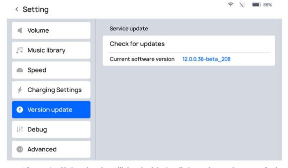
After tapping Update, the robot will download the installation package and a prompt for the download percentage prompt will appear. Once the download is complete for the installation package, the robot will automatically restart.
