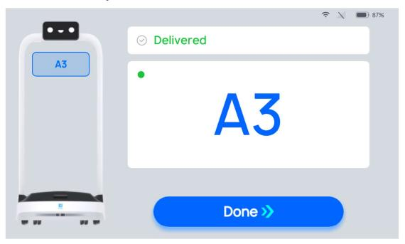
During the process of Direct, if you need to edit a task, force complete, cancel all tasks, or return, you can tap the robot's screen to pause the robot before proceeding with the operation. If there are no operations during the countdown period, the robot will continue running.
