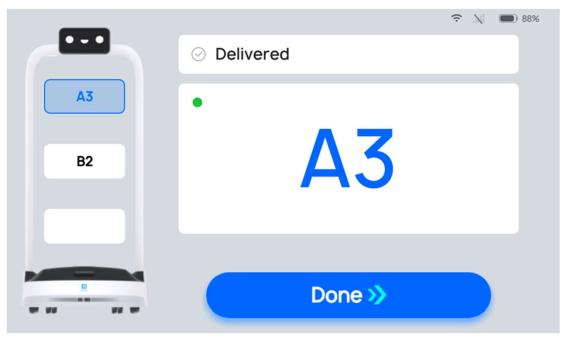
During the food delivery process, if it is necessary to edit a task, force complete, cancel all tasks, or return, you can tap on the robot's screen to pause the robot before proceeding with the
